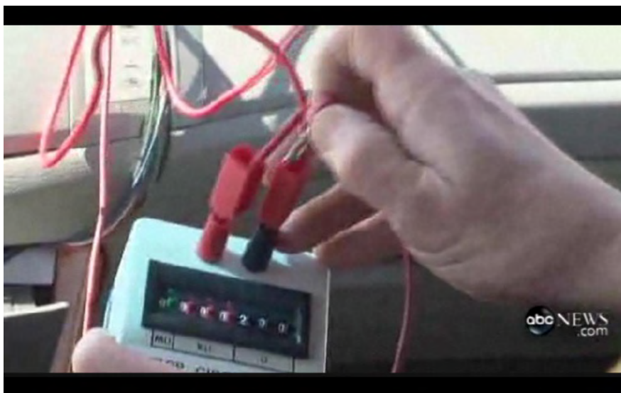
Figure 1. A 200-ohm resistance is apparently connected between the output signals of the two pedal position sensors. A third wire is about to be inserted into one side of the resistance.
